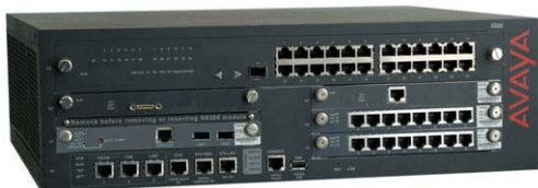
Figure 3: Sample H.248 system with installed modules
